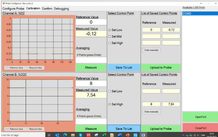
The screenshot shows the 'Configure Probe' window with two channels. Channel A (%O<sub>2</sub>) has a Reference Value of 0 and a Measured Value of -0,12. Channel B (%CO<sub>2</sub>) has a Reference Value of 8 and a Measured Value of 7,54. Both channels have 'Set High' selected under 'Select Control Point'. The 'List of Saved Control Points' is empty. The 'Available USB Ports' list shows 'COM3'. Buttons for 'Measure', 'Save To List', and 'Upload to Probe' are visible for both channels.
