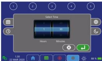
7. Rotate hour and minute wheels to place the actual time in the light blue bars.
