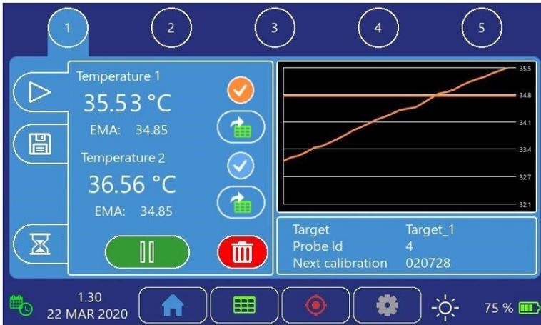
The measure window shows the continuous measurement value, in this example temperature.
