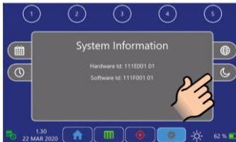
11. The NiloChecker can shut down automatically to save energy. Rotate time wheel to select time from last interaction, to shut down.
